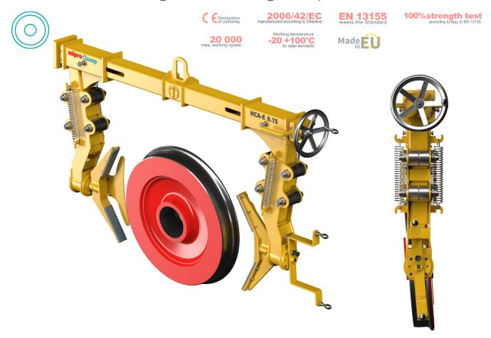
The clamp is intended for lifting railway wheels Before starting the lifting operation, the handle should be pre-tightened with a crank to a torque ~ 50 Nm, which is equivalent to 400 N on the crank handle
